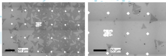
Figure 1. High resolution photo of the WS 2 flakes on our chip, with high magnification, taken under microscope. Flakes are about 25 microns wide.
